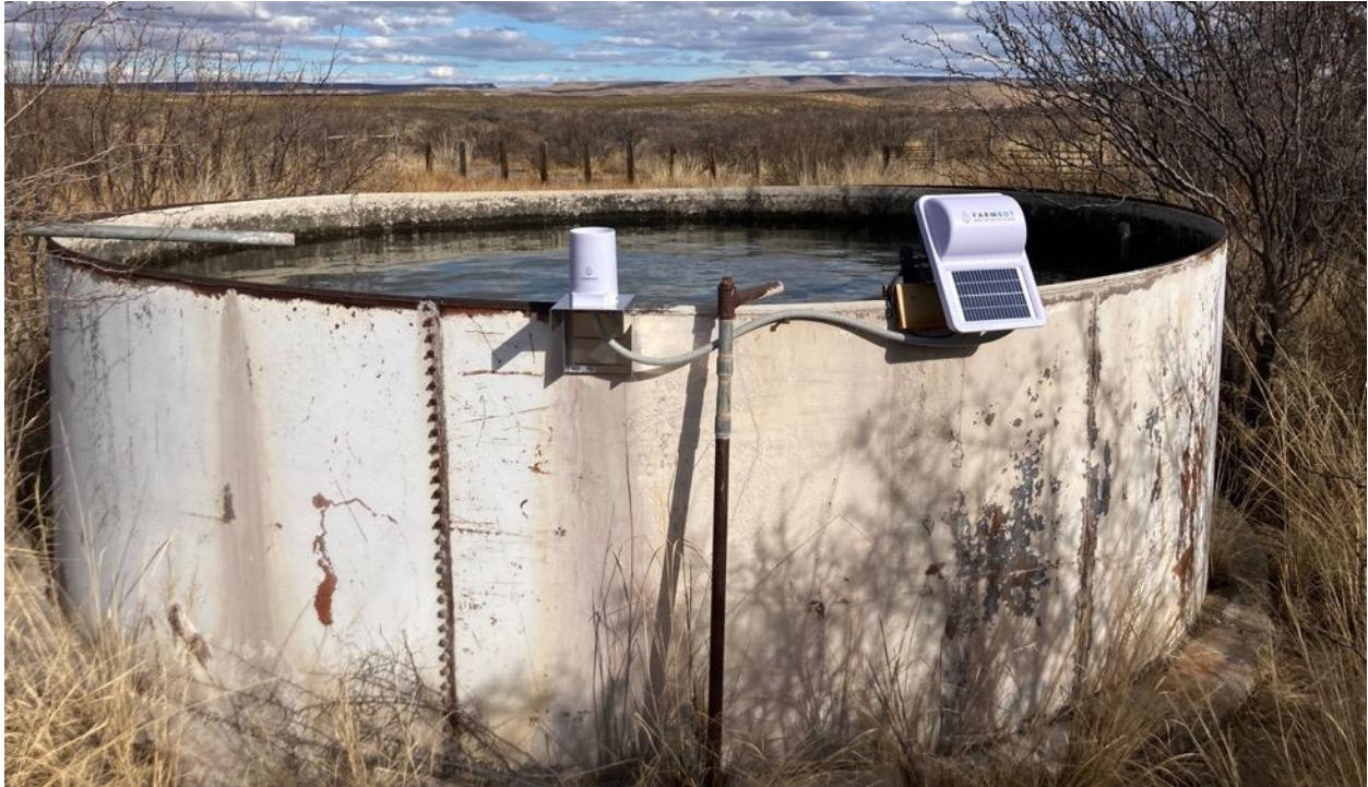
Figure 15. RanchBot rain gauge (left) and solar-powered tank sensor (right) installed at the Matanoso Pens of Alamito Creek Preserve, spring 2022 (Photo by Philip Boyd)
